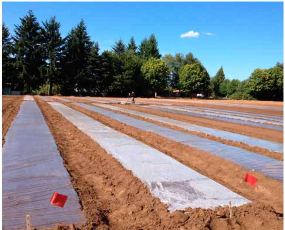
Figure 3. 2015 field trial comparing different types of solarization films. Note differences in clarity of anti-condensation (left) vs. regular plastic (right). Anti-condensing plastic achieved higher soil temperatures than did regular plastic.
